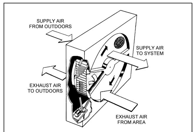
**Fig. 13 Rotary Air-to-Air Energy Exchanger**
