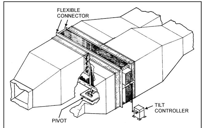
Fig. 20 Heat Pipe Heat Exchanger with Tilt Control
