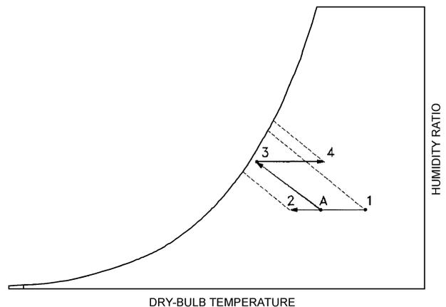
Fig. 10 Indirect Evaporative Cooling Recovery (Example 5)
