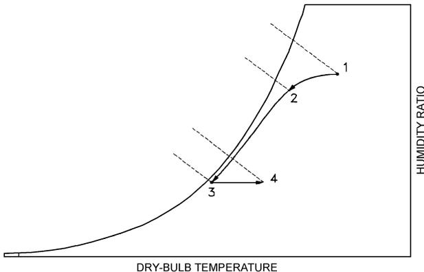
Fig. 11 Precooling Air Reheater Dehumidifier (Example 6)
