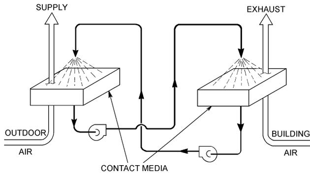
**Fig. 21 Twin Tower Enthalpy Recovery Loop**
