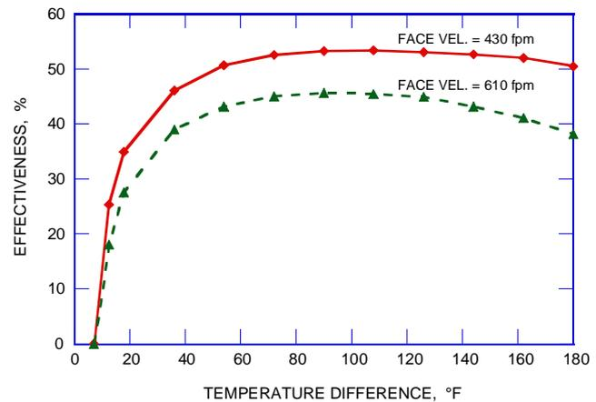
**Fig. 24 Typical Performance of Two-Phase Thermosiphon Loop**
