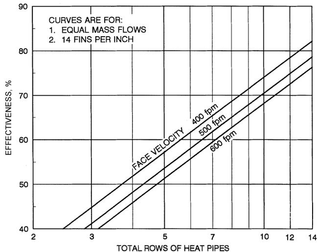
Fig. 19 Heat Pipe Exchanger Effectiveness
