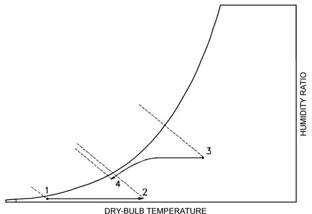
Fig. 8 Sensible Heat Recovery in Winter with Condensate (Example 3)
